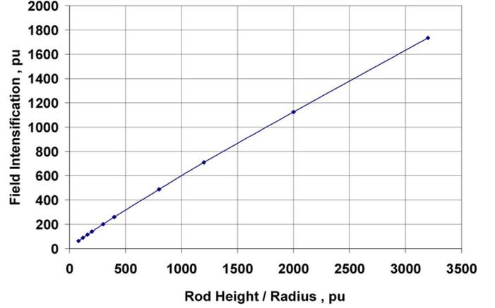
Fig. 1. Variation of the field intensification factor on the rod height to radius ratio. Hemispherically capped rod in the uniform field.
