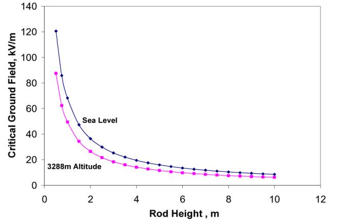
Fig. 2. Variation of the critical ground field for corona inception  $E_{gci}$  with a height of 2-cm diameter rod at different altitudes.
