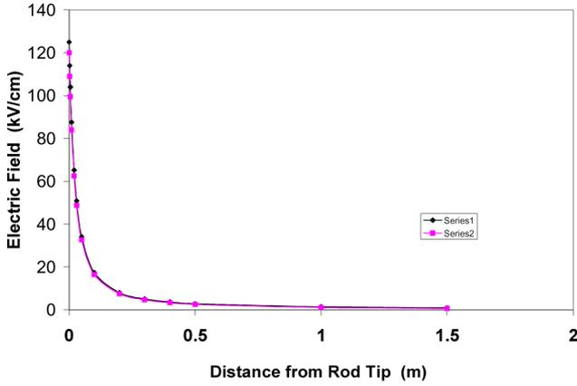
Fig. 4. Variation of the axial electric field with distance from the tip of the hemispherically capped 10 cm diameter rod. S1:30 m lightning mast on ground plane,  $E_g = 33.33$  kV/m. S2: 30 m rod-plane gap,  $U = 1000$  kV.
