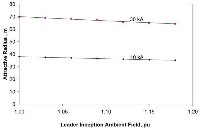
Fig. 8. Attractive radius of a 10 m rod to a negative descending leader: Effect of the relative increase in the critical upward leader inception field, caused by the space charge in the vicinity of the rod tip due to the cloud charge field ( $E_{gm} = 20$  kV/m) prior to the negative leader descent.
