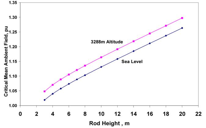
Fig. 7. Variation  $E_{gc}/E_{gc0}$  due to the corona space charge with a height of a 1 cm-diameter hemispherically capped lightning rod.  $E_{gm} = 20$  kV/m, at different altitudes.
