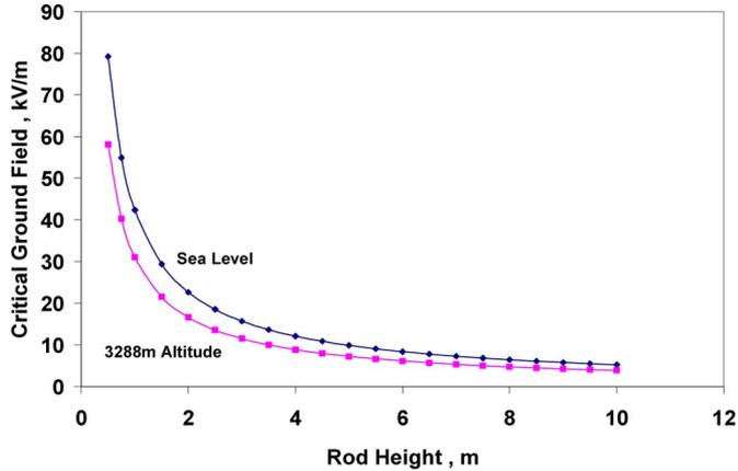
Fig. 3. Variation of the critical ground field for corona inception  $E_{gci}$  with height for a 1 cm diameter rod at different altitudes.
