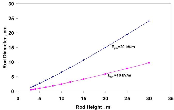
Fig. 9. Variation of the dc-corona free Franklin rod diameter with the tip height above ground for two levels of the maximum ground field due to cloud charges.
