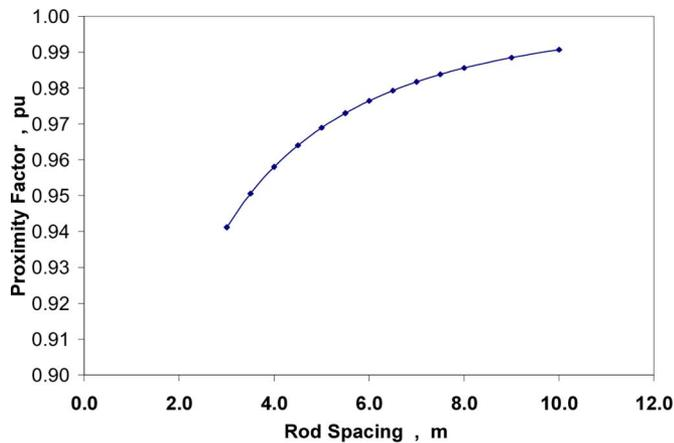
Fig. 11. Ambient field proximity factor due to an adjacent 6.4 m rod as a function of rod spacing.
