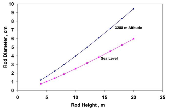
Fig. 10. Dependence of the required rod diameter for the dc-corona free performance on the rod height at different altitudes. Maximum ground field: 10 kV/m.
