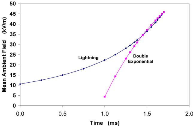
Fig. 5. Variation of mean ambient field in which a 30 m mast is immersed with time during negative leader descent and comparison with double exponential impulse of 3.6 ms front. Initial leader height: 500 m, radial distance: 89 m.  $I = 31$  kA, leader speed:  $2 \times 10^5$  m/s.
