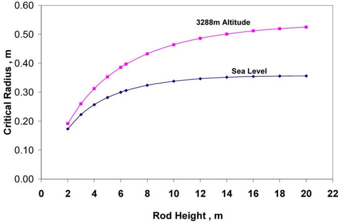
Fig. 6. Variation of the critical radius for upward leader inception of a hemispherically capped rod with rod height above ground at different altitudes.
